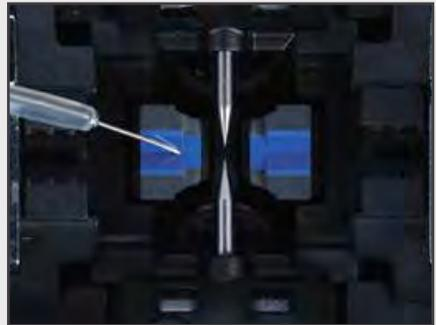
Test with fiber after cleaning with foam swab
