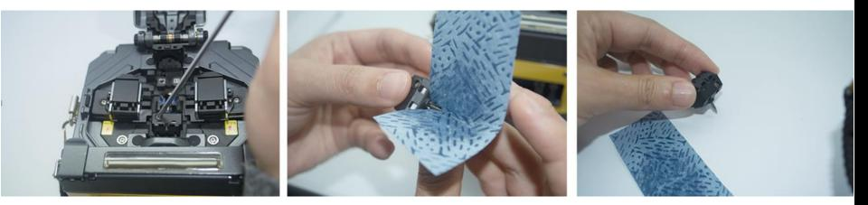
**4.** Remove electrodes carefully with a screwdriver 5.
